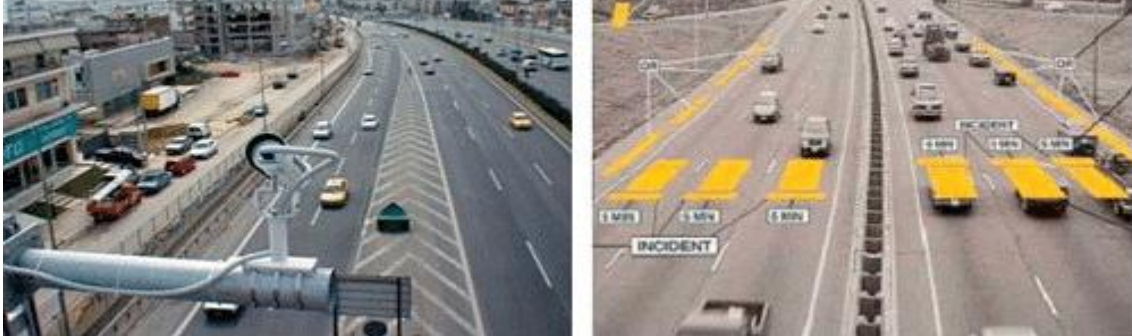
Left - normal traffic image | Right - a VIPS image with detection zones ( source )
